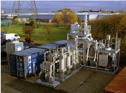
250 kg/h fast pyrolysis plant for liquids 250 kWe dual fuel diesel engine
