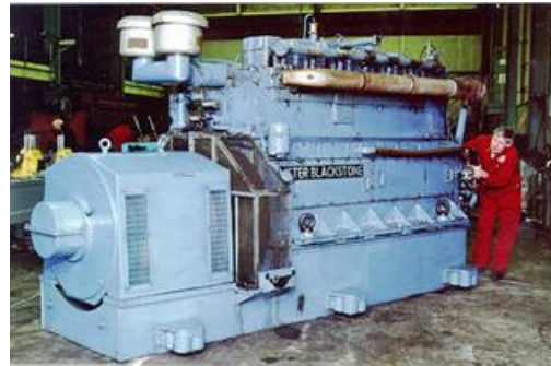
250 kg/h fast pyrolysis plant for liquids 250 kWe dual fuel diesel engine
